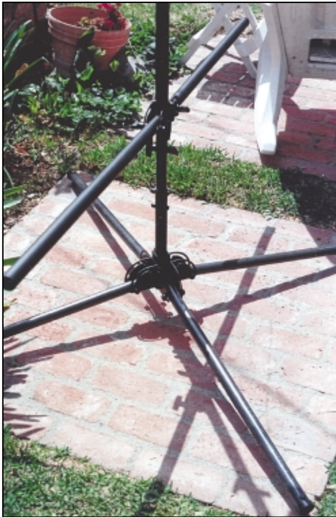
This is the optional “Quadpod” portable base for the Traveler antenna. Also visible is the lower dipole element, just a foot off the ground.
