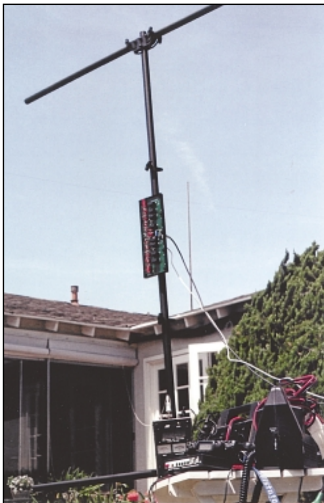
The TW-2010 set up and on the air for testing, with the coil/relay box open. Note the control cable and feedline coming away from the box at an approximately 45-degree angle. This is essential for keeping the SWR low (see text for details).
