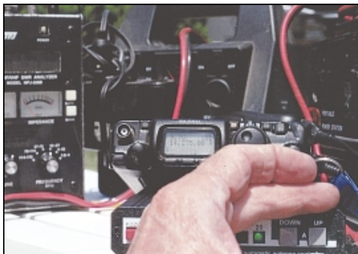
The green LED on the control box (shaded by Gordo's hand so you can see it in the bright sunlight) shows that the relays rest on 20 meters with the controller turned off. The up/down buttons are used to select the other bands, and the LED switches to indicate which band is in use.
